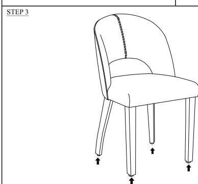
Turn clockwise or anti-clockwise to adjust leg leveller.
