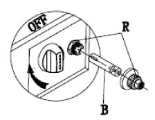
Remove the Electronic Ignitor Cap (16) on the electronic Ignitor (16) by unscrewing and slide the Battery (B) into the battery slot (16).
