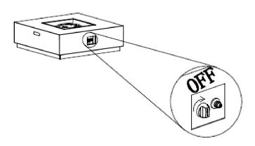
1. Check that the Control Knob (15) for the gas supply system is turned to the "OFF" position before starting any assembly.
