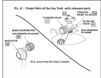
Pic. A: Shows the Charge Valve of the Cylinder with the different Valves and Coupling Nut, these forms the top of the Gas Cylinder.
