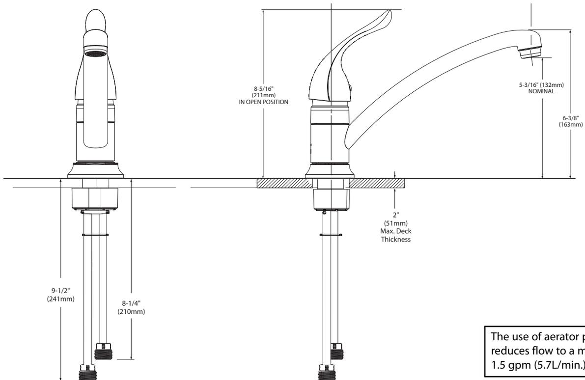
The use of aerator part 116711 reduces flow to a maximum of 1.5 gpm (5.7L/min.)
