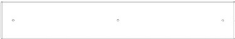
Y01 COVER BOARD - W4L20042 (x2) 5/8"x4"x24 3/16" (16x102x614)
