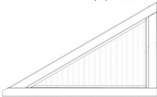
WA01 WINDOW ASSEMBLY - W2A04327 (x2) 1 7/16"x15 11/16"x24 3/4" (36x398x629)
