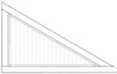
WA02 WINDOW ASSEMBLY - W2A04328 (x1) 1 7/16"x15 11/16"x24 3/4" (36x398x629)
