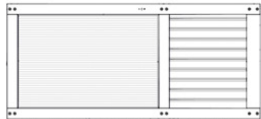
DA01 DOOR ASSEMBLY - W2A04072 (x1) 1 7/8"x36 9/16"x80" (48x928x2032)
