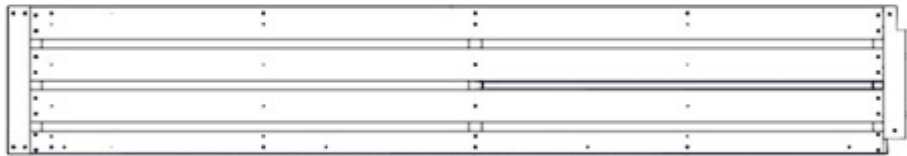
TB01 TABLE ASSEMBLY - W2A04325 (x1) 2 1/16"x14 7/8"x89 1/2" (52x378x2274)
