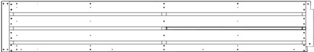
TB01 TABLE ASSEMBLY - W2A04325 (x1) 2 1/16"x14 7/8"x89 1/2" (52x378x2274)
