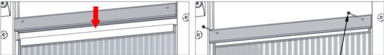
SLIDE GROOVE IN WINDOW CAP OVER WINDOW ASSEMBLY AND SCREW INTO PLACE.
