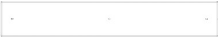
Y01 COVER BOARD - W4L20042 (x2) 5/8"x4"x24 3/16" (16x102x614)
