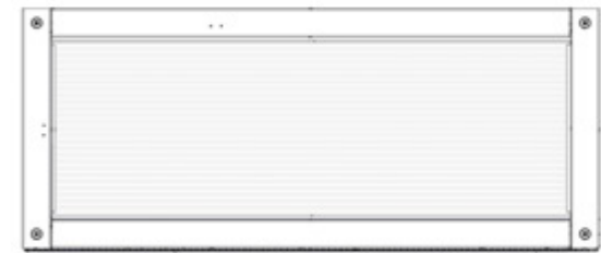
WA03 WINDOW ASSEMBLY - W2A04330 (x1) 1 7/8"x19 5/8"x47 3/16" (48x498x1198)
