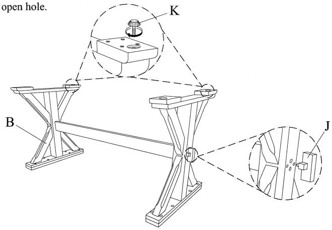
5 Place Table Top(A) upside down on soft surface. Align and fasten Trestle Leg(B) to Table Top(A) using JCBC Bolt(E), Spring Washer(G) and Flat Washer(H) and fully tighten with Allen Wrench(L).
