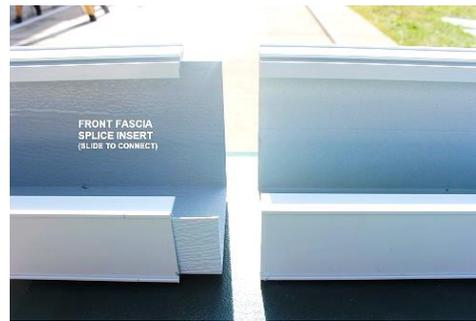
**STEP 3:** Connect 2<sup>nd</sup> piece into other end of splice insert piece end to match STEP 1 center mark from other side. Secure with white Tek screws from bottom exterior.
