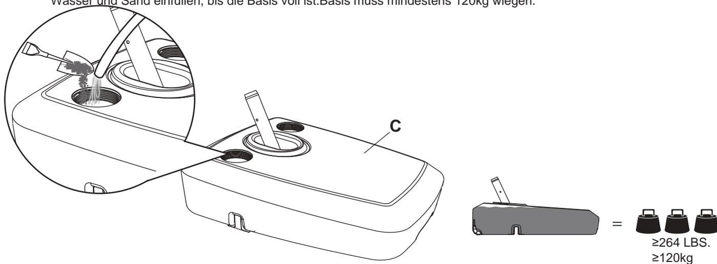
7 Tighten the Plastic Cap (E) on the base.
