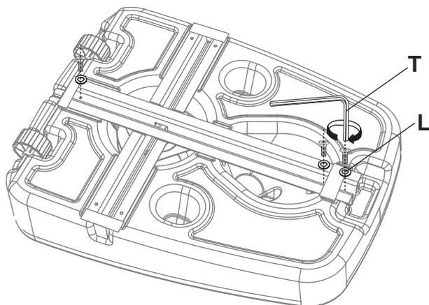
6 Insert water and sand until base is full. Base needs to weight more or equal to 264LBS.
