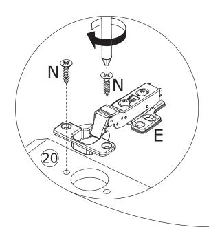
Fix hinge(E) to panel 20 with screw(N) as shown.
