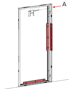
Figure 12. Drilling a hole.
