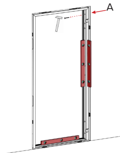
Figure 13. Installing an anchor.
