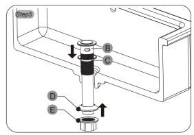
Follow step 2 and 3 to install D, E onto B (C is no need in this process), if there is any further issue, please feel free to contact us (support@gele.ltd) for help.
