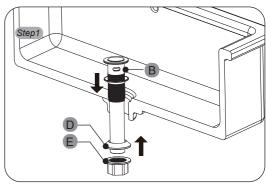
Remove parts D and E from the drain, insert B into the basin hole, and then install D and E on B in sequence.
