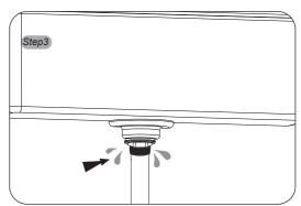
Check whether leakage happened here under the basin sink; You need apply some silicone to prevent leakage issue if there is leaksge under the basin sink, Follow steps 4 and 5 to apply the silicone and complete installation;
