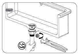
Use a wrench to tighten the fasten nut (E).
