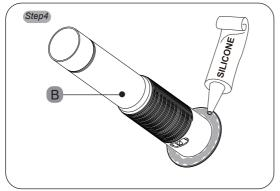
Remove C,D and E from B, apply the silicone to underside of flange as shown. Insert B into sink hole;
