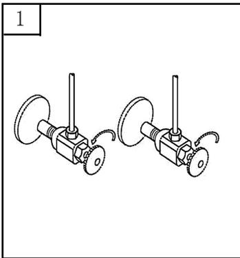
1. Shut off water supply. Remove old faucet. Clean sink surface in preparation for new faucet.
