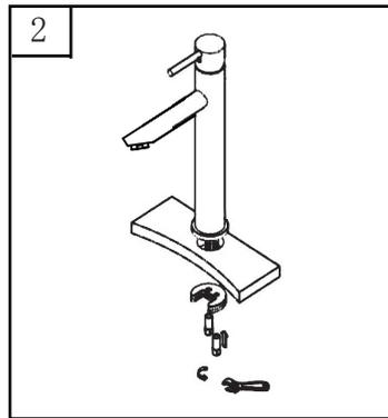
2. Screw cold/hot copper tube onto faucet body.
