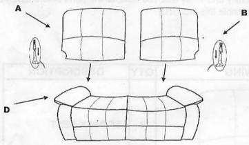
Step 2. Attach the ears to the back rest, insert the ears and push to the end, make sure the brackets is secured in position.
