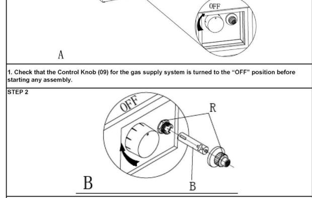
Remove the Electronic Ignitor Cap (11) on the electronic Ignitor (11) by unscrewing and slide the Battery (B) into the battery slot (11).
