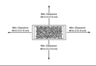
Keep the appliance area clear and free from combustible material, gasoline and other flammable vapors and liquids.
