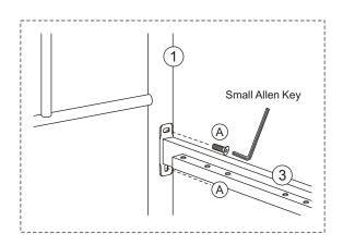
$\underline{\textbf{IMPORTANT:}} \ \ \textbf{Do not tightly secure the screws before completing Step 2}.$
