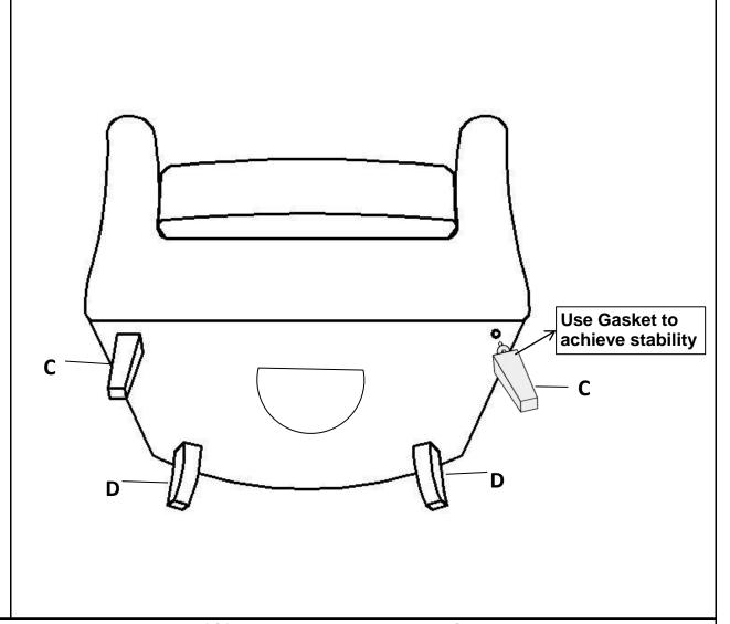
Install the Front Wooden Leg(C) at the bottom of the Sofa by placing one Gasket(1) on the threaded stem.
