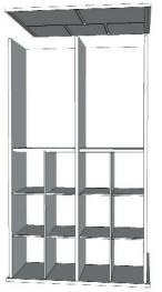
**Step 11:** Install Right Side Panel so that edge of assembled pieces fit firmly into mortises and back grooves. Insert hex screws into pre-drilled holes in Right Side Panel. Tighten down halfway.
