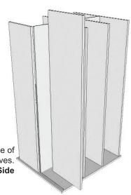
Step 9: Insert Back Bottom Panel into mortise of Left Side Panel. Make sure to align back grooves. Insert hex screws into pre-drilled holes in Left Side Panel. Tighten down halfway.
