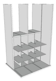
Step 7: Insert Front Small Divider ¼" into mortises of Top Panel and Front Shelf Panel or Front Bottom Panel and Front Shelf Panel aligning notches in the Front Center Divider. Repeat for remaining Small Divider ¼".
