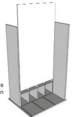
**Step 8:** Insert sides of Back Panel into back grooves of Top Panel. Slide down until edge rests firmly in back groove of Left Side Panel.
