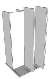
Step 8: Insert Back Shelf Panel into the mortises of the Left Side Panel. Insert hex screws into pre-drilled holes in Left Side Panel. Tighten down halfway.
