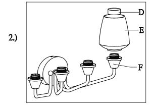
Step 2. Attached the glass(E) on the socket then secure by socket ring(D).
