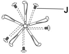
Connect the leg (G) and the base (F) with screws (J)
