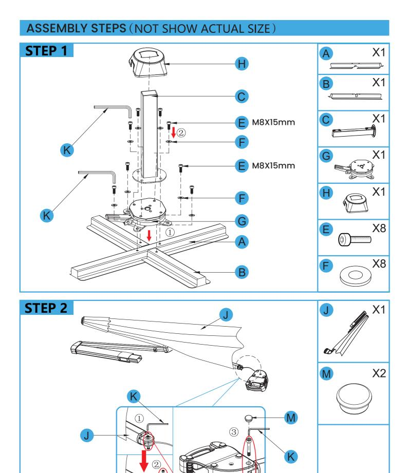
Notice: This screw and nut come from the cantilever, not from the hardware accessory package.
