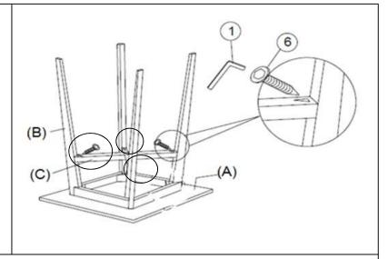
Align the support leg (C) and support leg (D) into the mortise leg (B) as shown above.
