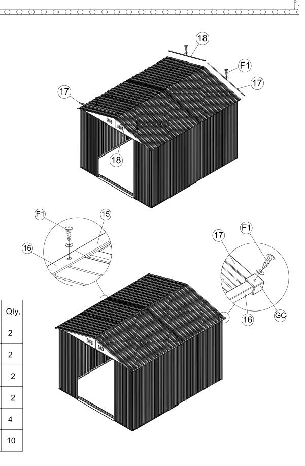
Place two pieces of the roof flashing center (19) on top of the roof panels, Line up the holes and secure them with (F1) screws with washers. Then slide the flashing end cap (GE) to the front & back top of the roof and secure with (F1) screws with washers. See figures below.
