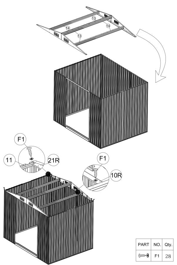
Place the roof panels (P5),(P6)and (P7) on the top of Gable panel (21L), Line up the holes and secure with (F1) bolt, and nut with washers. Then place the roof panels secure them with (F1) screws with washers.
