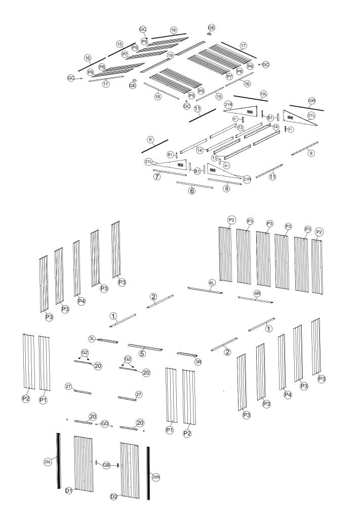
Assemble base bars from (1) to (4R) with (F1) Screws. Then place the entrance taper channel (5)on top of the bar(3L) and(3R). Secure with (F1) screws to the foundation. Seeing the following figures .Make sure the base bar assembly in a perfect square.
