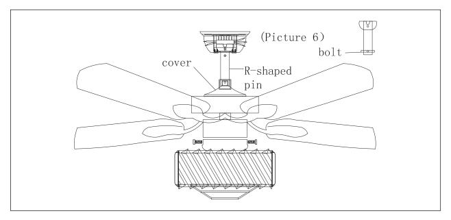
2.Put the ceiling fan on the mounting bracket and slowly rotate the ceiling fan until the slot position of hanging ball is at the correct place. (See Picture 7 & 8)
