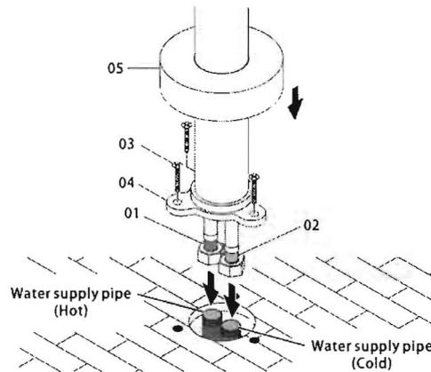
Step 9 (Figure A). Insert rubber washer (02) to hose (01) and thread them to the handshower bridge.
