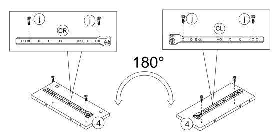
Attention: The hole positions are different when installing the slide on the front and back of the board 4.
