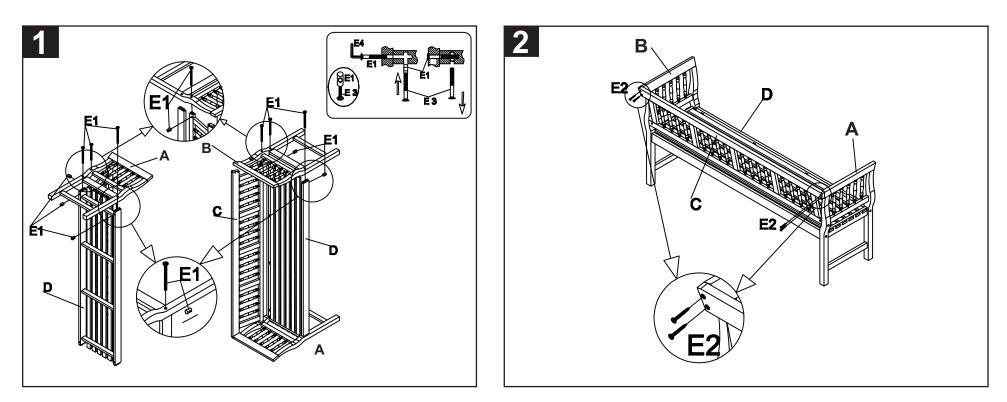
Step1: attach the right side (A) and the left side (B) to the seat (D) as shown on the picture by using the Allen bolt (E1) and tighten all with the Allen key (E4). Make sure you don't tighten the side too tight. This you will do at the end.
