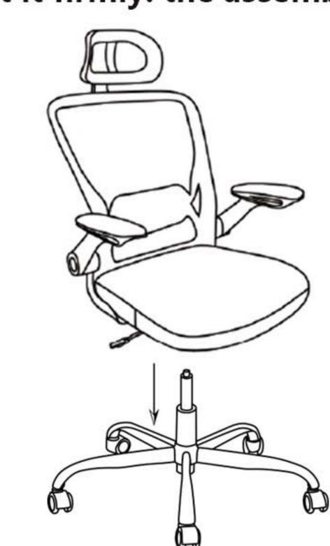
\* Caution: If the Air Rod (5) doesn't insert to Base Plate (7) firmly, it's likely to fall off when the chair raises up.
