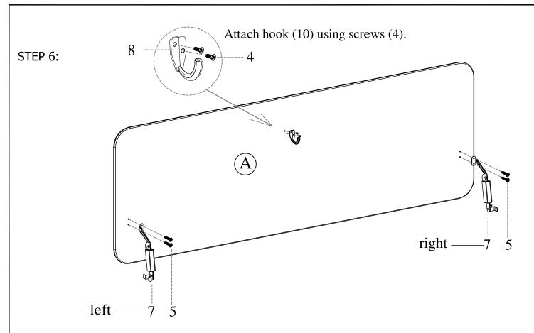
Attach left and right safety hinge (7) to top panel (A) using screws (5).
