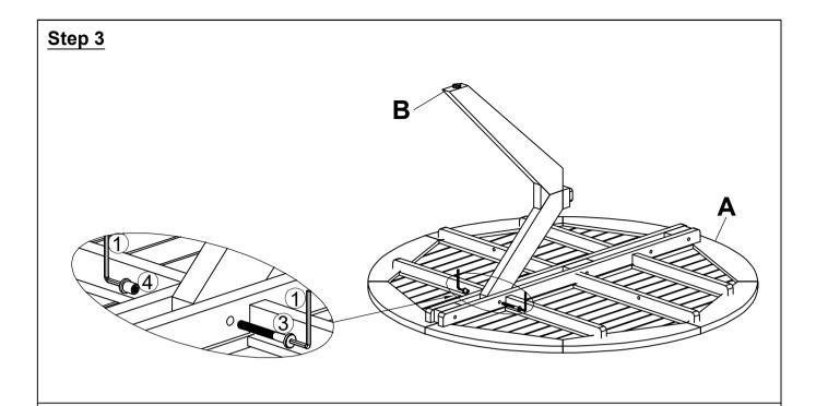
Position the First Leg (B) as shown above picture. To affix the First Leg (B) to the Table Top (A), using Bolt (③), Sleeve Nut (④) and 2 Allen Wrench (①) as above picture. **Do not fully tighten the Bolts.**
