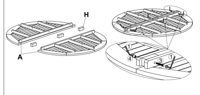
To affix the two halves of the Table Top together, align the bolts mounting position of the Table Top (A) to the mounting position of the Block (H). Insert the Bolt (③) through the mounting position and affix the Table Top using Sleeve Nut (④) and 2 Allen Wrench (①), as shown as above picture.
