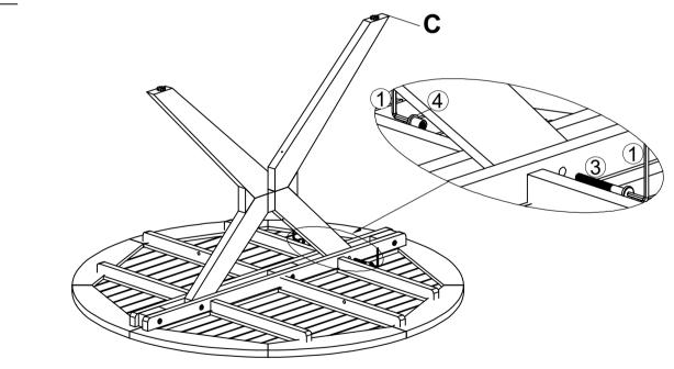
Repeat the same process as Step 3 to affix Second Leg (C) to Table Top (A), using Bolt (③), Sleeve Nut (④) and 2 Allen Wrench (①) as shown above picture. **Do not fully tighten the Bolts.**
