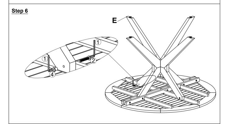
Repeat the same process as Step 5 to affix Fourth Leg (E) to Table Top (A), using Bolt (2), Sleeve Nut (4) and 2 Allen Wrench (1) as shown above picture. **Do not fully tighten the Bolts.**
