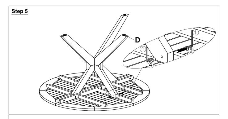
Position the Third Leg (D) as shown above picture. To affix the Third Leg (D) to the Table Top (A), using Bolt (2), Sleeve Nut (4) and 2 Allen Wrench (1) as above picture. **Do not fully tighten the Bolts.**
