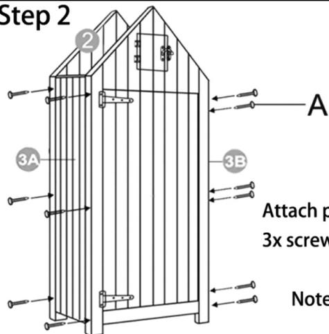
Attach part 3A to part 1 finished in step 1, secure with 3x screw (A); Attach part 2 to 3A, using 3x screw (A). Repeat for the right side panel part 3B using 6x screw (A).
