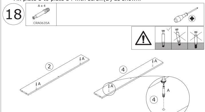
Insert quickfit screw(A) into plate 2 and 4 with a screwdriver as shown.
