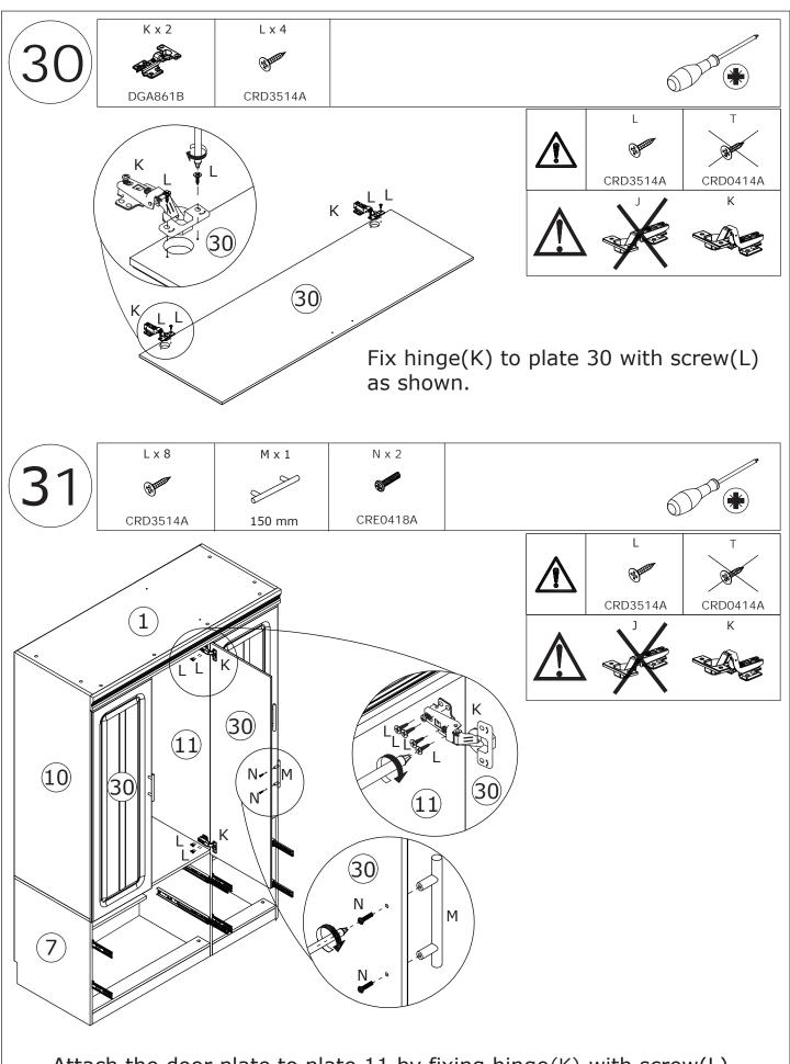
Attach the door plate to plate 11 by fixing hinge(K) with screw(L) as  $shown.Fix\ handle(M)$  with screw(N) as shown.
