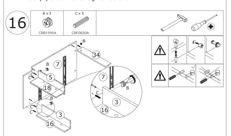
Insert wooden dowel(C) into plate 5,18,3,16 and 34 at first, attach to plate 7 as shown.
