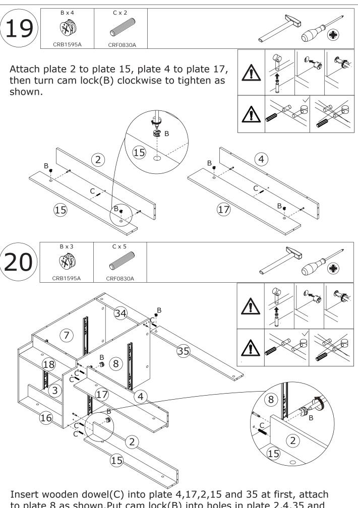
to plate 8 as shown. Put cam lock(B) into holes in plate 2,4,35 and turn clockwise to tighten as shown.
