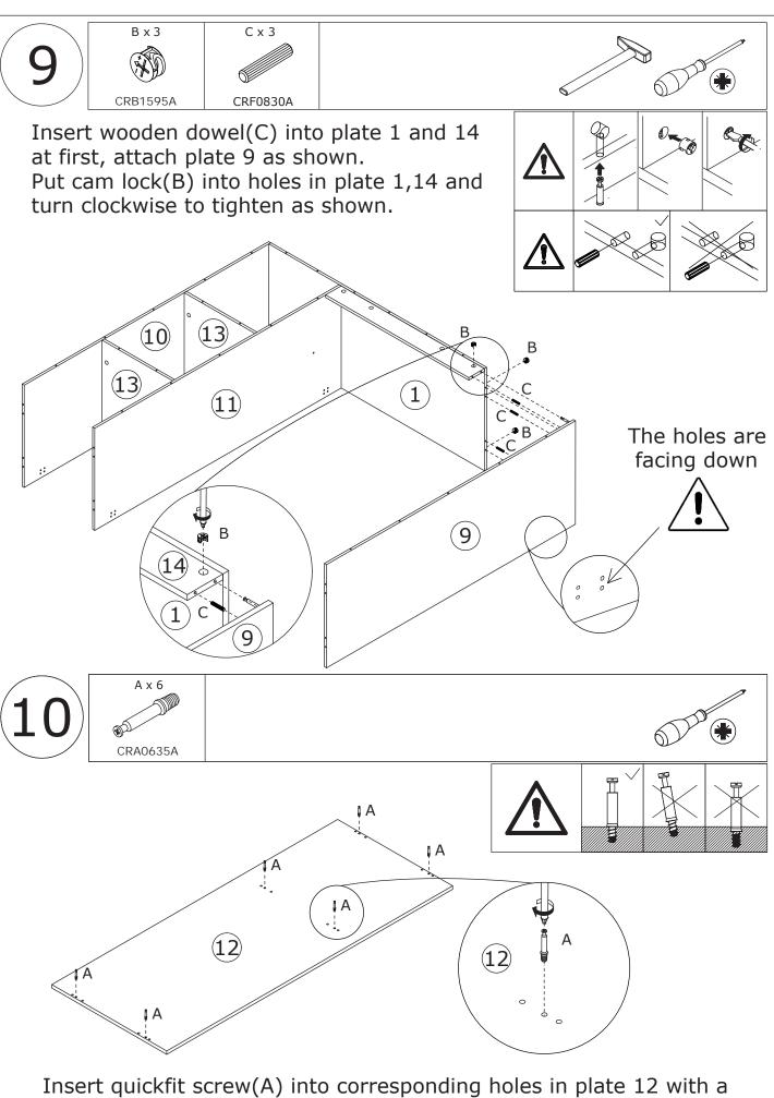
Insert quickfit screw(A) into corresponding holes in plate 12 with a screwdriver as shown. Please pay attention to the holes where the accessories are inserted.  $_{10/29}$
