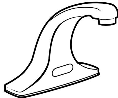
**Deck-Mount (4" Center), Non-Mixing, Battery Powered Electronic Faucet**
