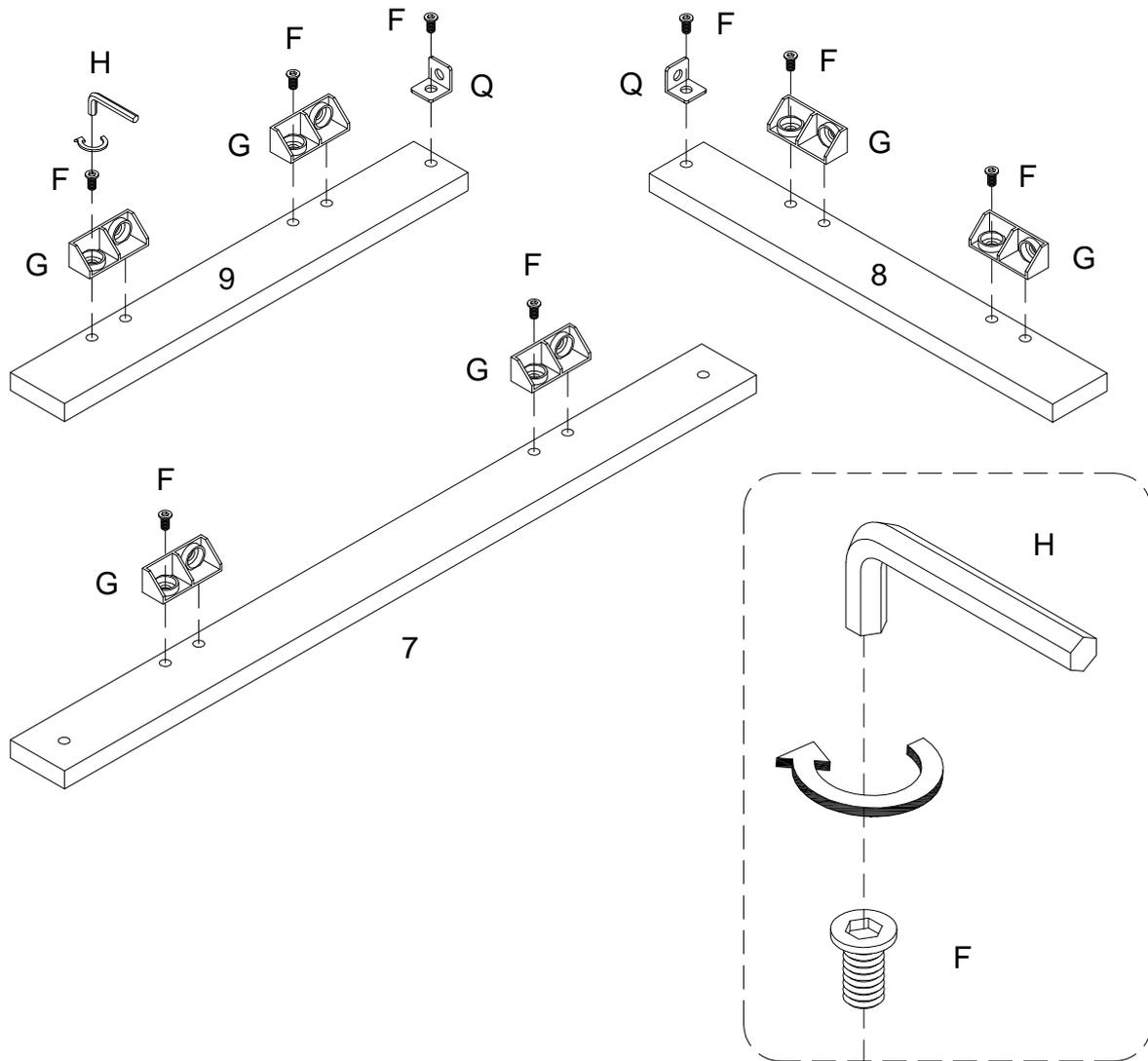
Using bolt (F) attach plastic wedge (G) into parts (7,8,9) ,then using bolt (F) attach connecting iron sheet (Q) to parts (8,9) with hex key (H) as per diagram.
