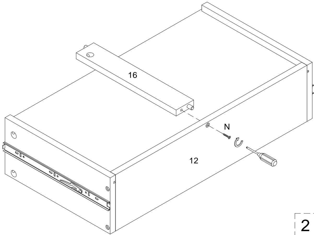
Using screw (N) secure part (12) into part (16) with Philips head screwdriver as per diagram.
