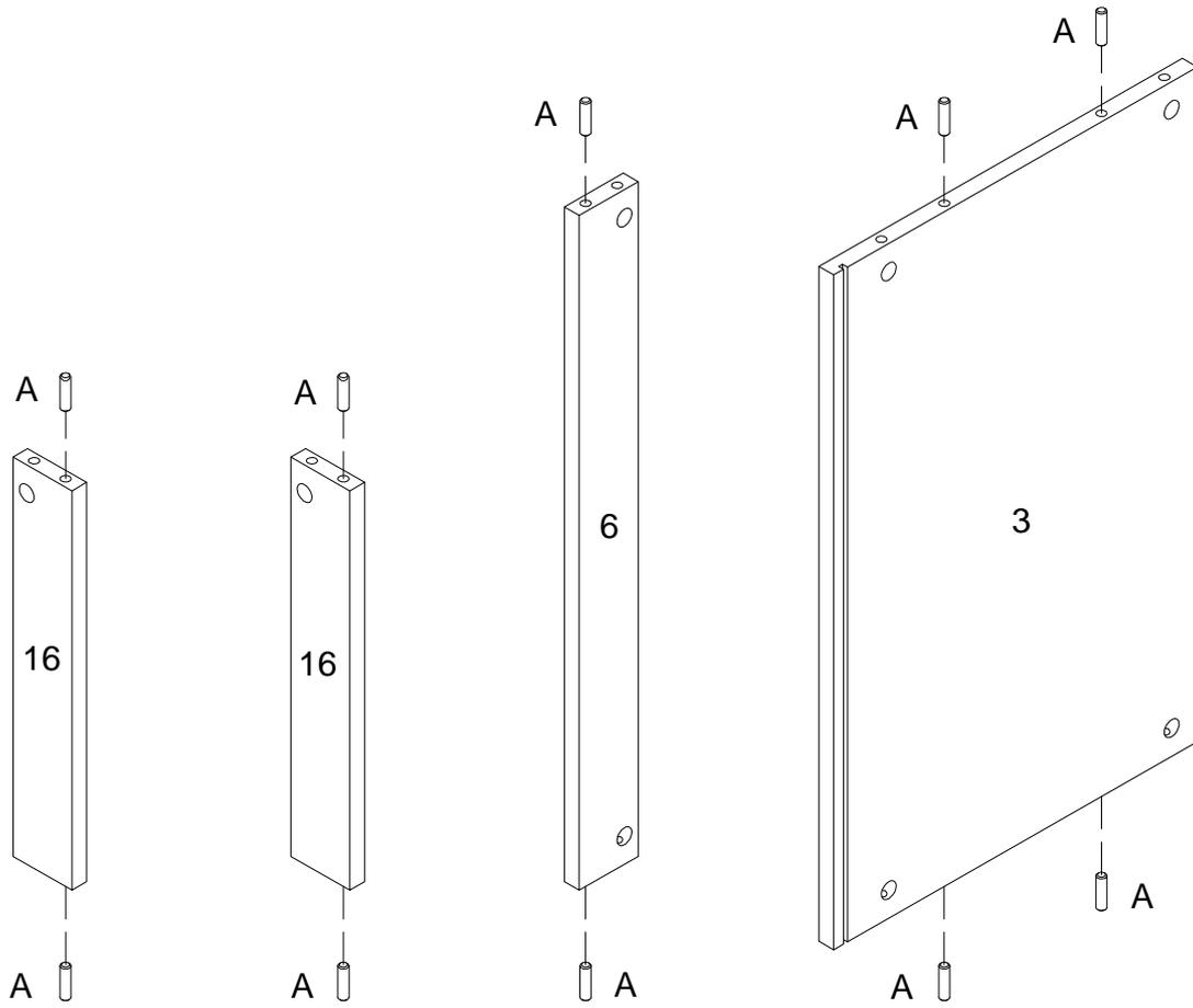
Insert wooden dowel (A) into parts (3,6,16) as per diagram.
