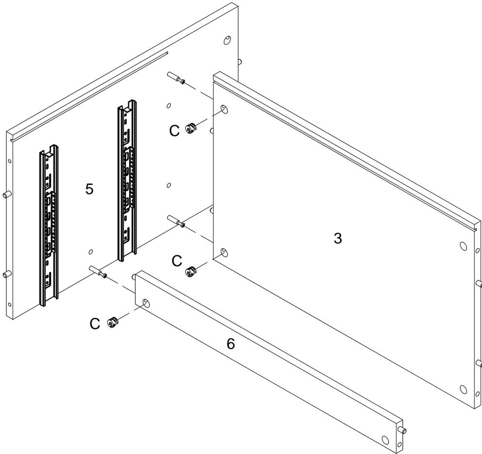
Using cam lock(C) secure parts (3,6) to part (5) with Philips head screwdriver as per diagram.
