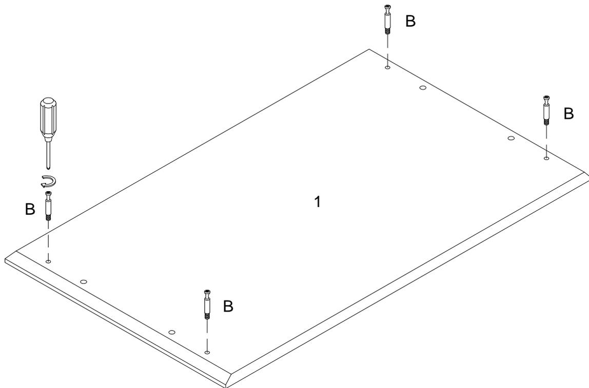
Secure cam bolt (B) to part (1) with Philips head screwdriver .
