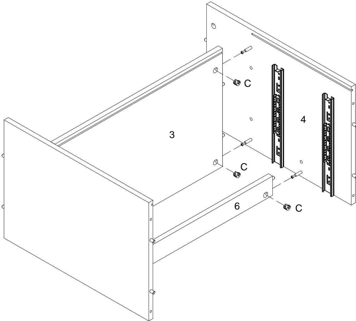
Using cam lock(C) secure parts (3,6) to part (4) with Philips head screwdriver as per diagram.
