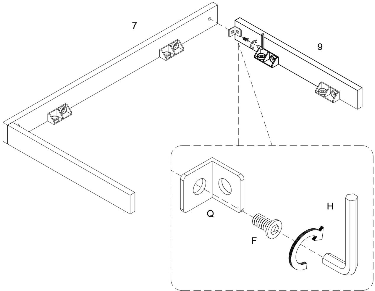
Using bolt (F) attach connecting iron sheet (Q) to part (7) with hex key (H) as per diagram.
