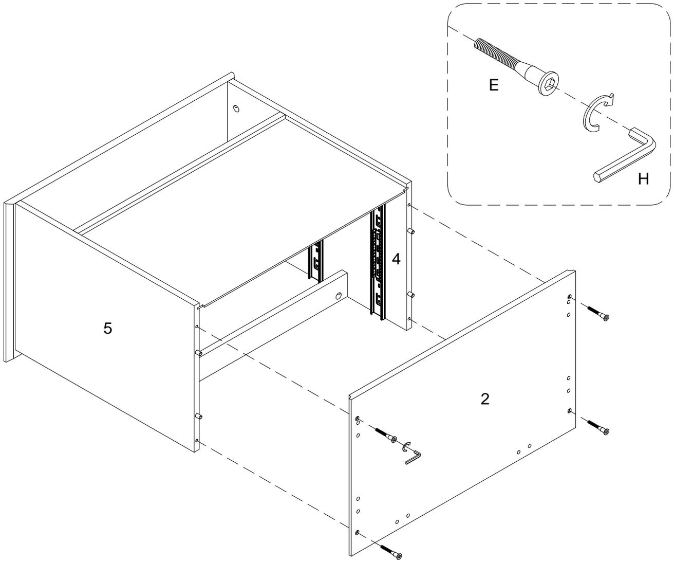
Using bolt (E) attach part (2) into parts (4,5) with hex key (H) as per diagram.
