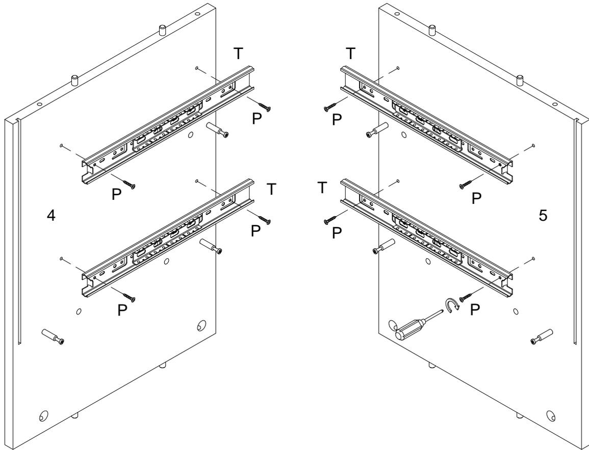
Using screw (P) attach drawer slider arm (T) to parts (4,5) with Philips head screwdriver as per diagram.
