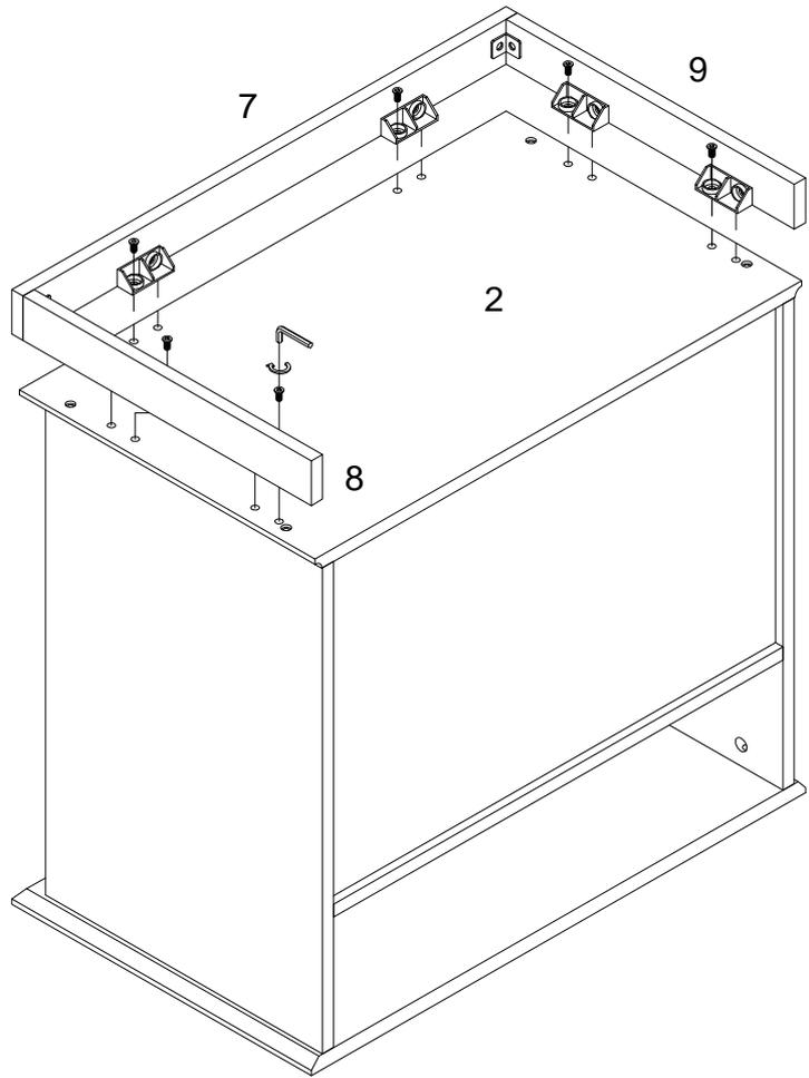
Using bolt (F) attach plastic wedge on parts (7,8,9) to part (2) with hex key (H) as per diagram.
