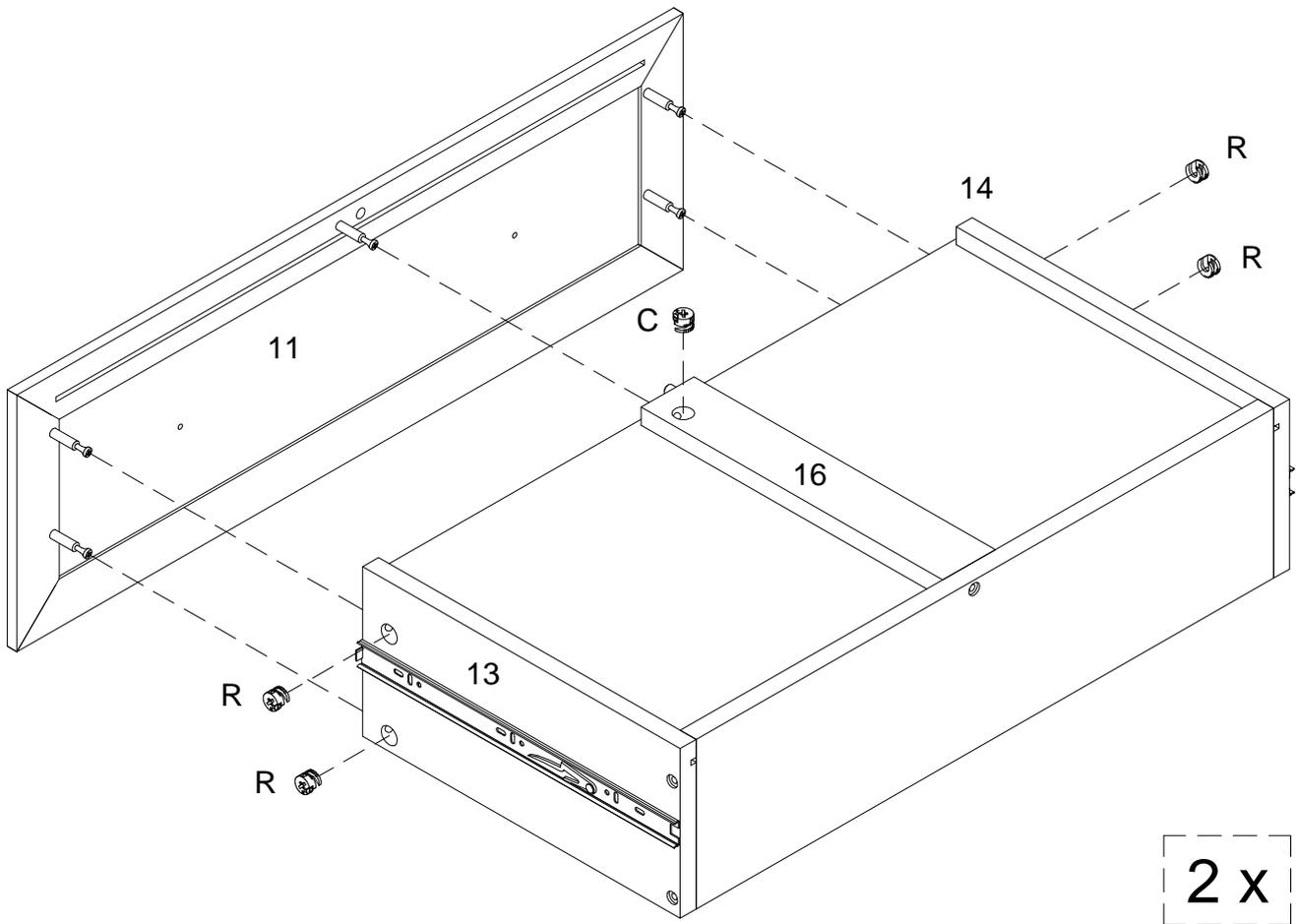
Using cam lock(R) secure part (11) to parts (13,14) ,then using cam lock(C) secure part (11) to part (16) with Philips head screwdriver as per diagram.
