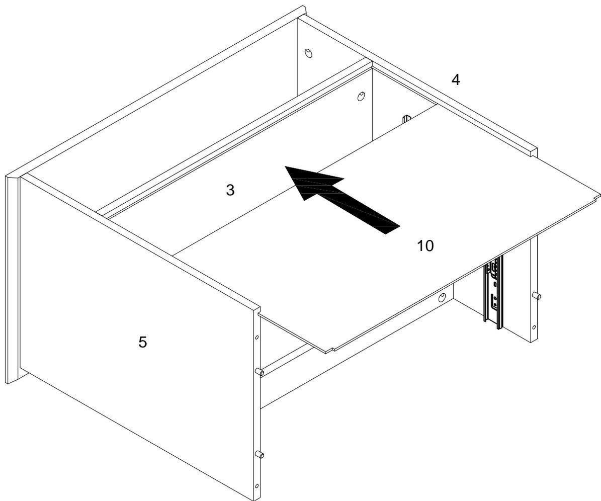
Put part (10) into parts (3,4,5) as per diagram.
