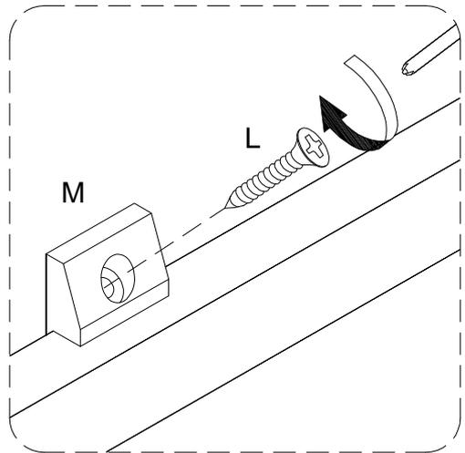
Using screw (L) secure plastic wedge (M) to part (10) with Philips head screwdriver as per diagram.
