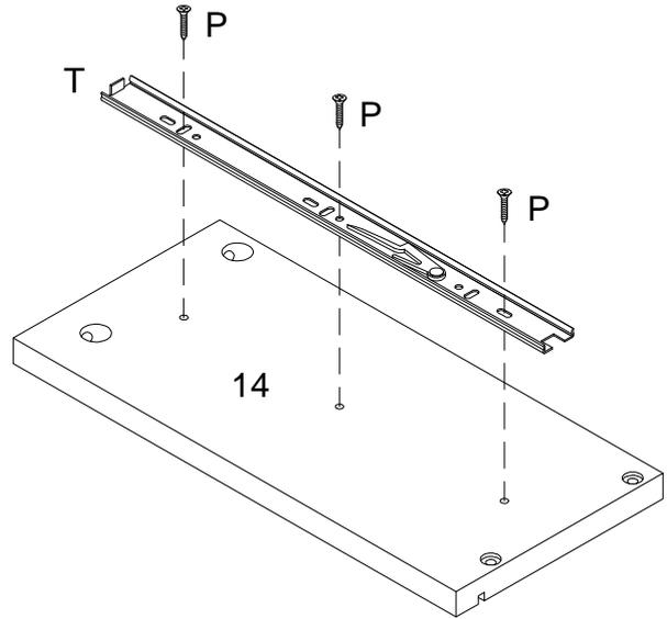
Using screw (P) attach drawer slider bracket (T) to parts (13,14) with Philips head screwdriver as per diagram.
