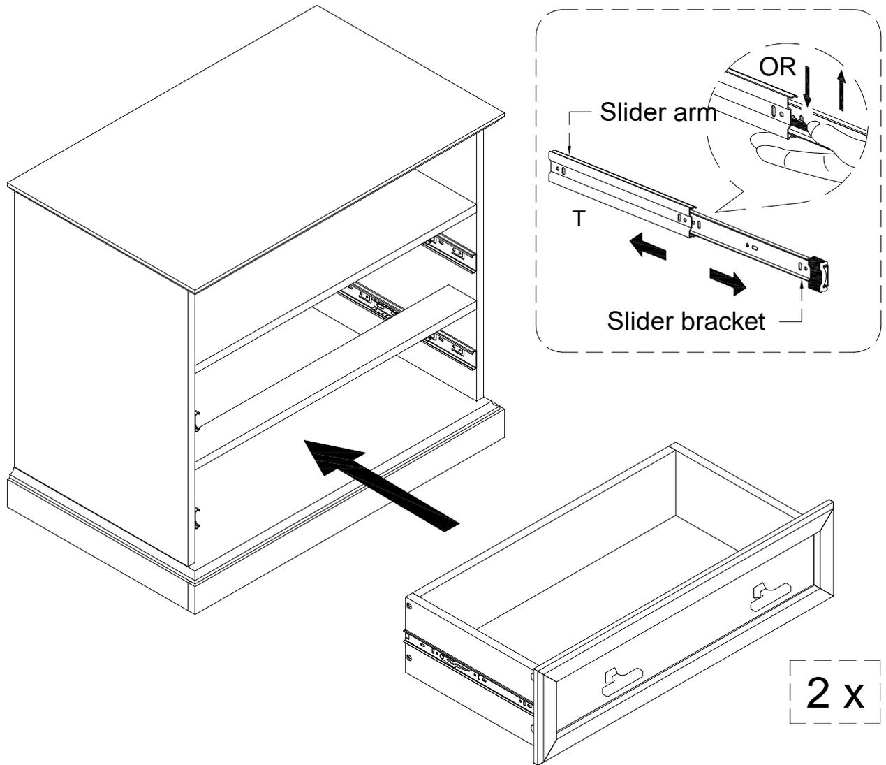
Put slider bracket into slider arm as per diagram .
