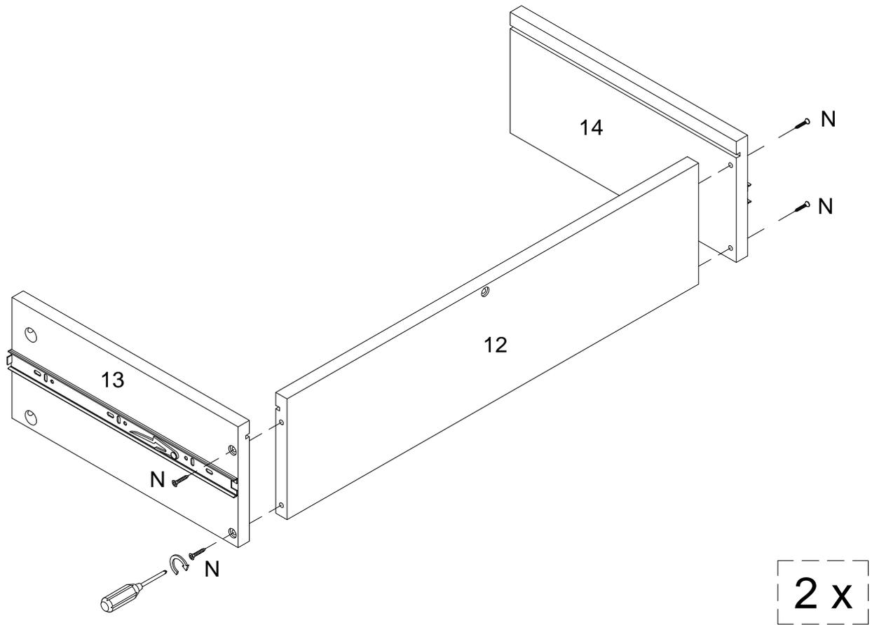
Using screw (N) attach parts (13,14) to part (12) with Philips head screwdriver as per diagram.
