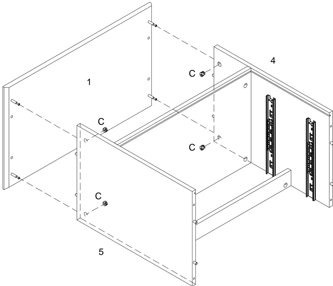
Using cam lock(C) secure part (1) to parts (4,5) with Philips head screwdriver as per diagram.
