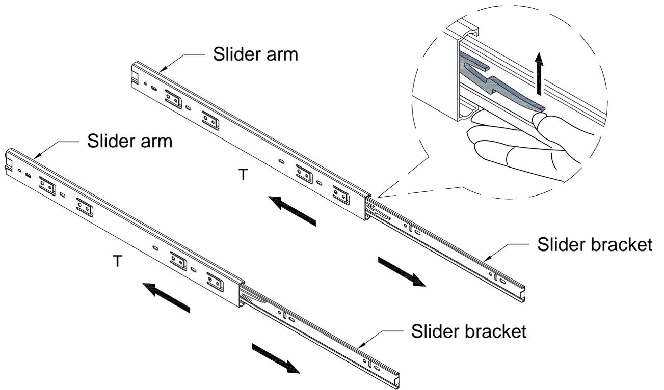
Pull out the slider bracket from the slider arm as per diagram.
