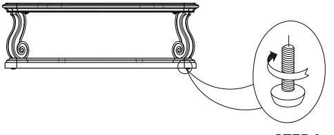
Adjust Leveler if needed to level table on uneven floor.
