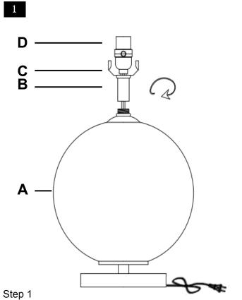
Pull power cord to connect the Neck (B) to the Base (A).
