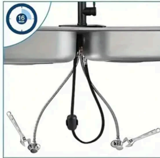
4. Connect water line to angle valve by wrench
