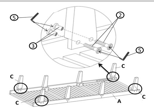
Position Side Leg (C) to Foldable Seat Panel (A) as pictured above. Affix the Side Leg (C) to Foldable Seat Panel (A) using Short Bolts (②), and Sleeve Nuts (③) with Allen Key (⑤).
