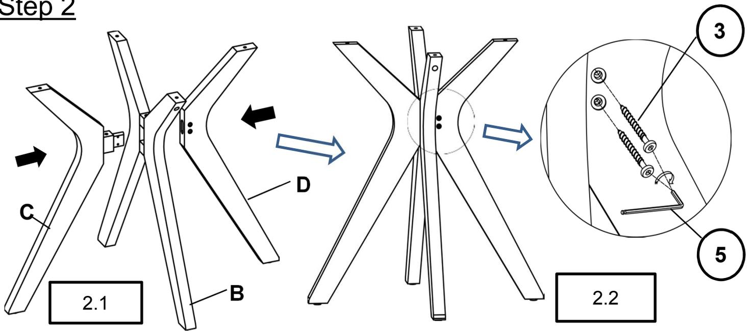
**2.1)** Insert Second Leg(C) and Third Leg(D) through the First Leg(B) as shown above.
