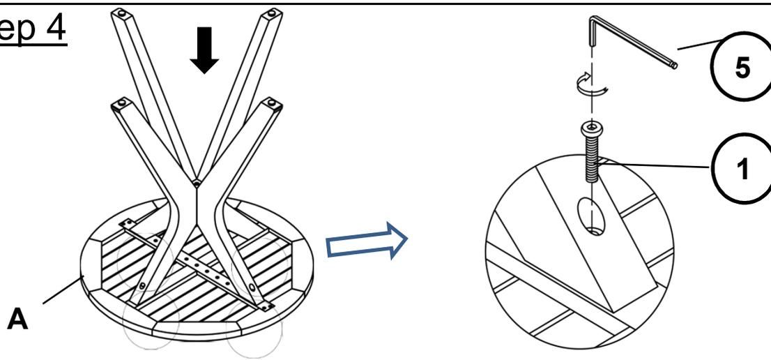
Attach Leg Frame to the Table Top(A) using Bolts(①) with Allen Key(⑤).
