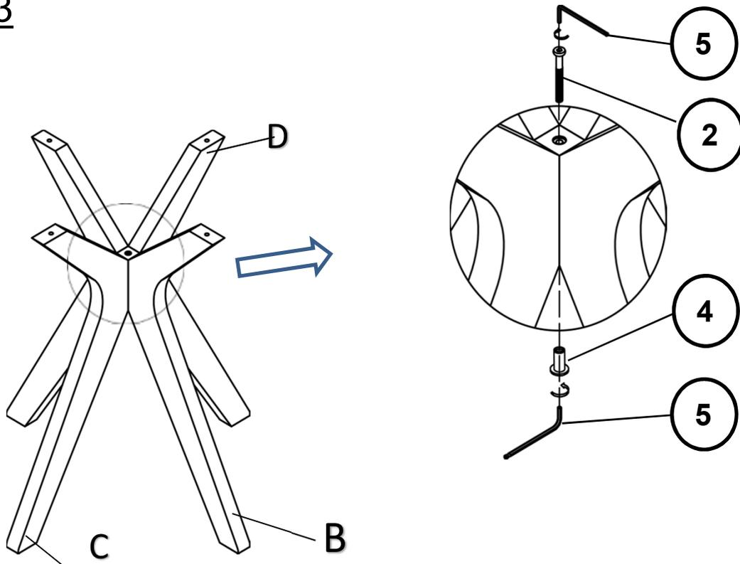
Then, attach First Leg(B) to Second Leg(C) and Third Leg(D) using Bolt(2) and Sleeve(4) with Allen Keys(5).
