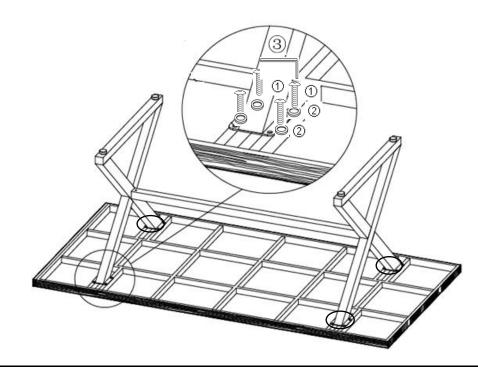
Turn the table top upside down to a soft surface to avoid scratching. Attach Table Leg with Pre-attached Levellers(B) to the mounting position on the table top(A) with Bolts(1), Washers(2) by Allen Wrench(3). **DO NOT OVERTIGHTEN.**
