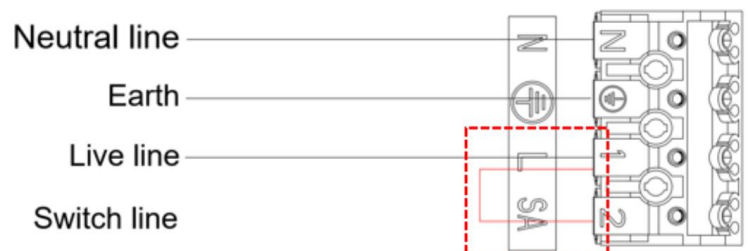
Emergency Luminaire wiring ② (Light will be 7 x 24h ON)
