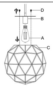
**Step 6:** Insert the bulbs (A) into the Sockets(B). Fix the Sockets (B) to the Lamp body(C) with Final Screw(D)
