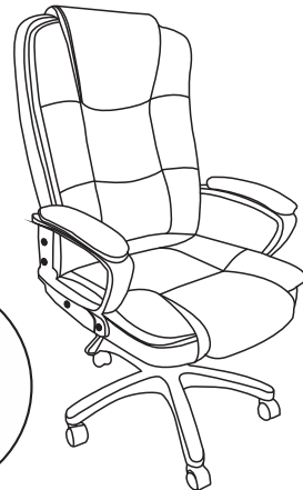
4.Rocking Adjustment Function The tighter the knob is turned, the less shaking it is, and vice versa.
