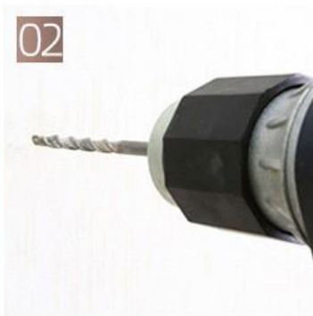
Use an electric drill to drill holes on the wall ( please use drill bit 6 )
