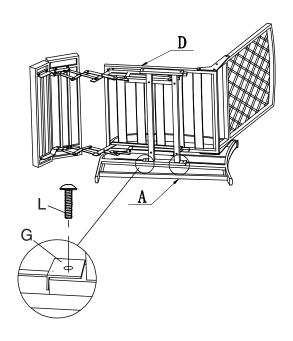
Connect Armrest (Part B) to Seat (Part D) using Washer (Part G) and Screws(J) as shown in diagram.
