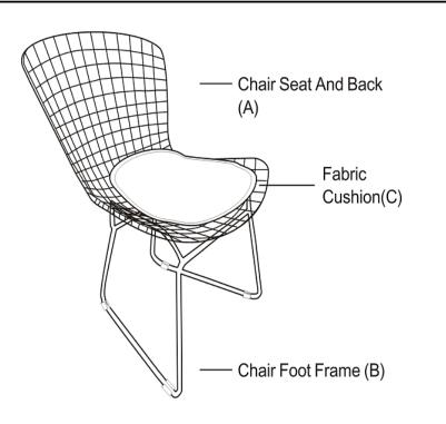
This Steel wire chair has multiple parts and may require up to 30 minutes to assemble. To give you an overview of the Steel chair parts, the above picture is to help you put the various parts into perspective. Please read through the instructions herebelow to familiarise the parts and steps before assembly.
