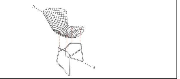
Place the Chair Foot Frame (B)onto a clean, soft surface to avoid any scratches or damages to the product, and then put the Chair Seat And Back (A) upper on the Chair Foot Frame (B).
