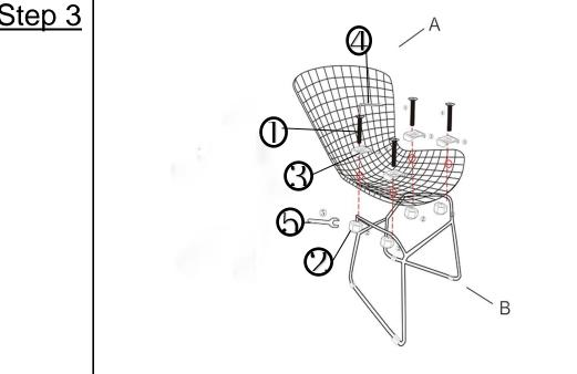
Fix the Chair Foot Frame (B) with Chair Seat And Back (A) by using Bolt (1), Pad(3), Hex Nut (2) use Allen Key(4) and Hex Wrench(5). Repeat the previous step and according to four red circles Mounting Position, Repeat the same process by affixing Bolts (1), (2), (3)to designated points, Each of the four red circles above can be assembled first.
