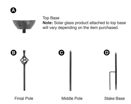
**Step 1:** Attach top base (A) to finial pole (B) by turning it to the right until it is firmly tightened.
