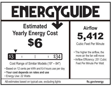
Energy information listed above is a weighted average of High and Low speeds tested with the downrod supplied.
