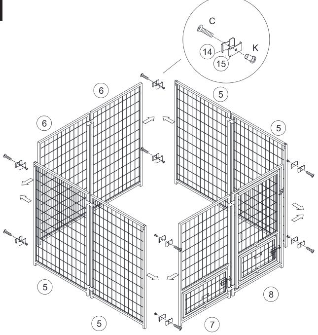
Screw the hardware C / K to the part 14/15 to connect each side as showing.
