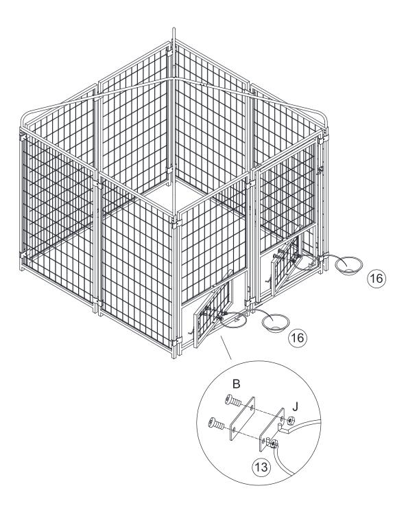
Fix the part 13 with hardware B/J as showing , and then put it on the part 16.
