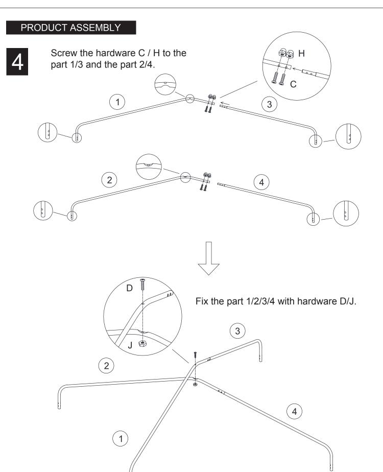
Fix the part 1/2/3/4 to the frame with hardware D/J as showing.
