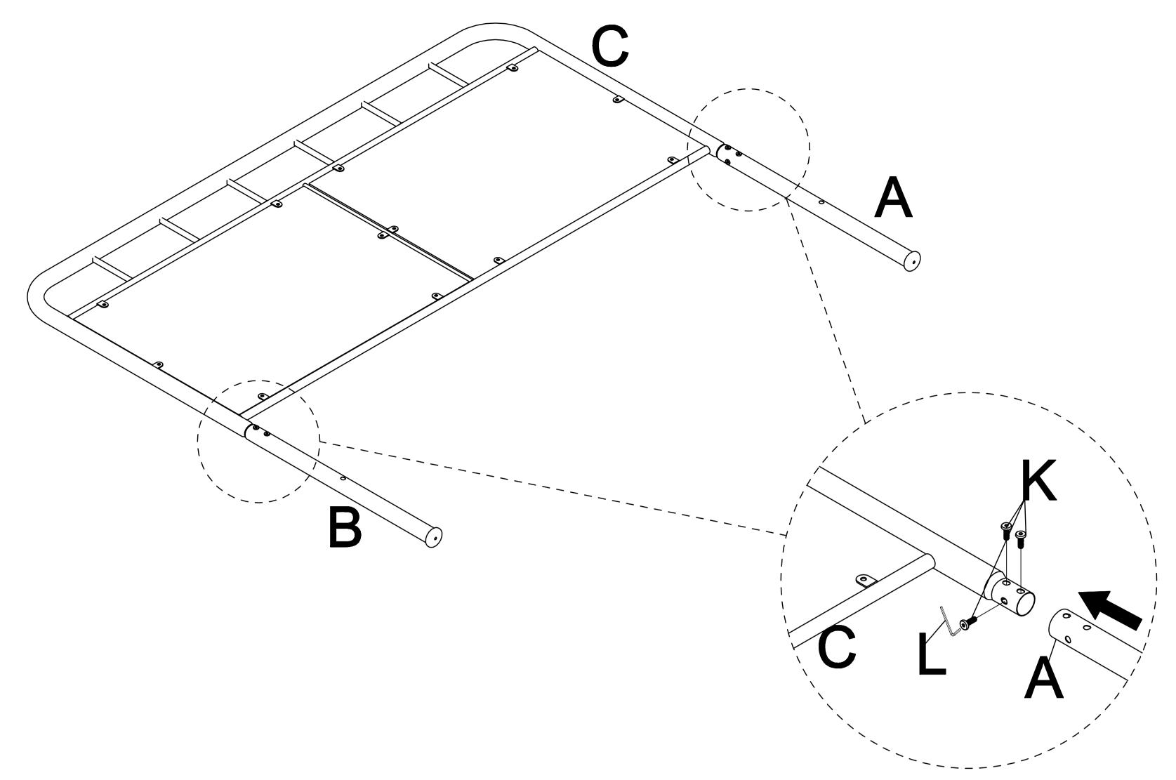
Insert the Rail Section (2) (F) to the Rail Section (1) (E), and then insert the Bolt (K), turn the L-Allen Key (L) to tighten them.
