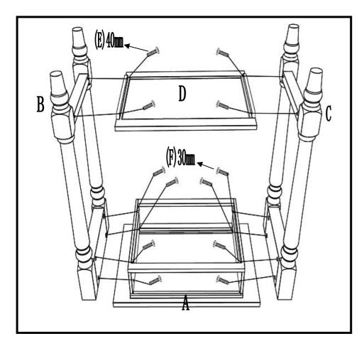
Turn the Top (A) upside down, attach the legs to top, use Allen Key to tighten the bolts (F). Then attach the Shelf (D) to legs, tighen the bolts (E)
