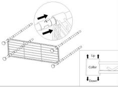
Pushing firmly down on every shelf at corners by rubber mallet to ensure the shelf in a place over the plastic clips and screw the leveling feet in or out to attain proper
