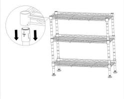
Please mare sure that you have the Wire Shelf(A) the correct way up, hold the wire shelf on it's side and slide the top of four lower poles through the bottom of the wire shelf at it's corners until there is a snug fit, and then set the wire shelf
